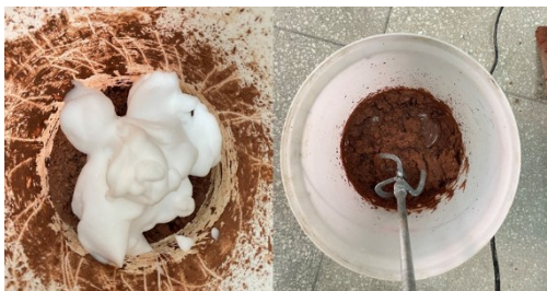
图4 改良泥岩制备过程 Fig. 4 Preparation process of improved mudstone
